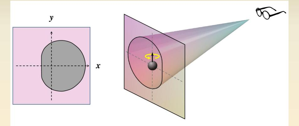
(1) Frequency dependence of the shadow position for circular polarized light;
